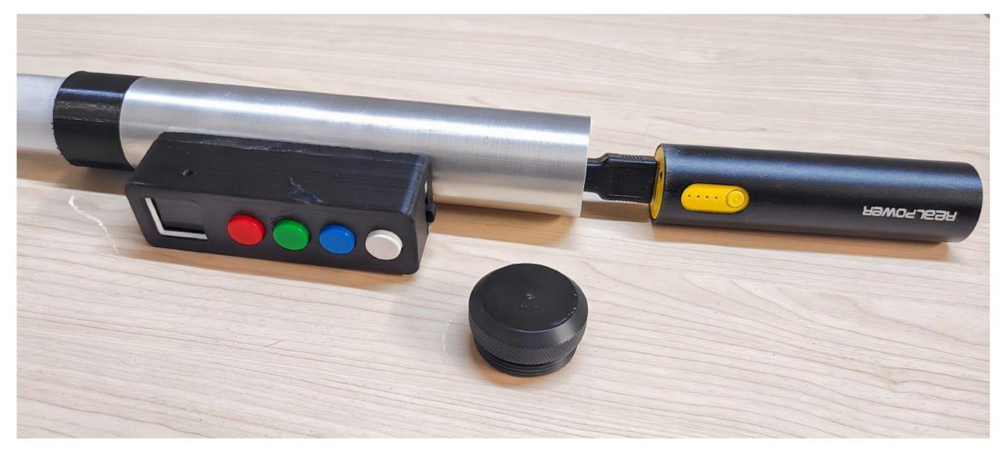
The power bank is charged with the included USB charging cable; the charging status is displayed via the LEDs on the power bank
